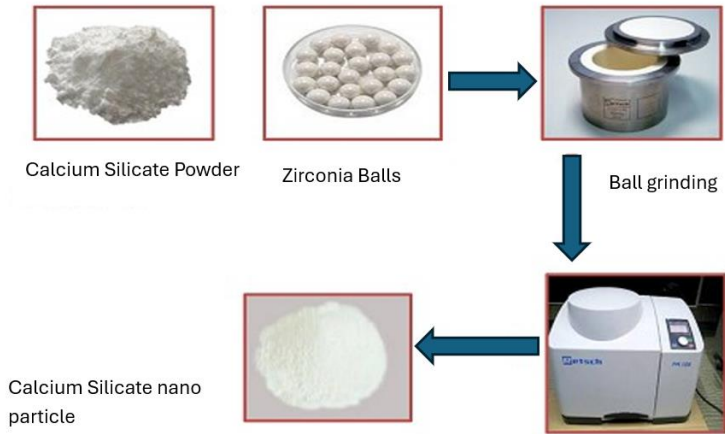
Figure 1: Silicate nano particle preparing method (Yadav, 2021)
