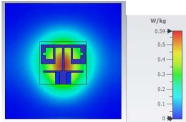
Fig. 10 Simulated SAR distribution of the proposed wearable antenna on the human tissue phantom at 2.45 GHz.
