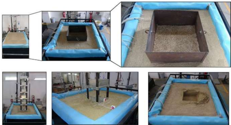
Figure 2: The building model and instrumentation, together with the various stages of experimental work Source: Erdiñçliler and Yildiz, 2023
