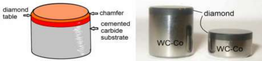
Figure 3. Sketch and photograph of polycrystalline diamond compacts, consisting of a sintered diamond layer or table located on a cemented carbide substrate (Lancaster et al, 2007:1), (Frushour & Torbet, 2001:1).
