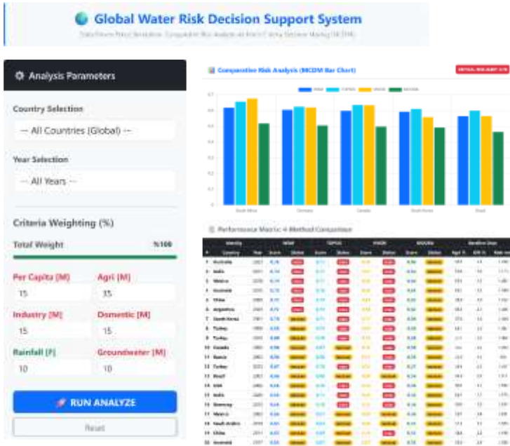
Figure 11 The interactive web interface of the Global Water Risk Decision Support System displays multi-method (WSM, TOPSIS, VIKOR, MOORA) risk comparisons and country-level filtering.
