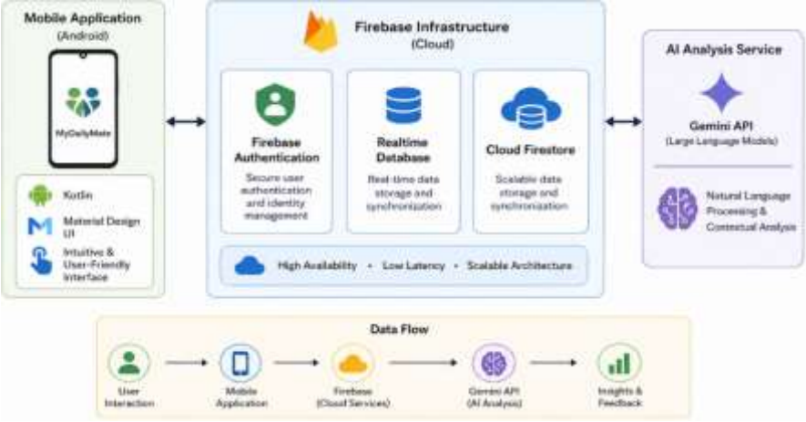
Figure 2. MyDailyMate Technological Infrastructure System and Components
