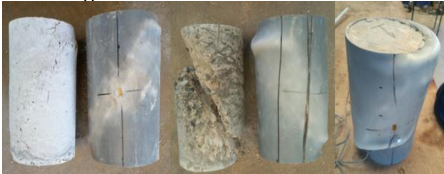
Figure 2: Compressive fracture of composite specimen (Woldemariam, 2019)
