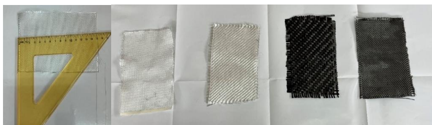
Figure 2. 100 mm x 150 mm glass and carbon fiber fabric samples cut to be used in the coating of sample panels and measurement control
