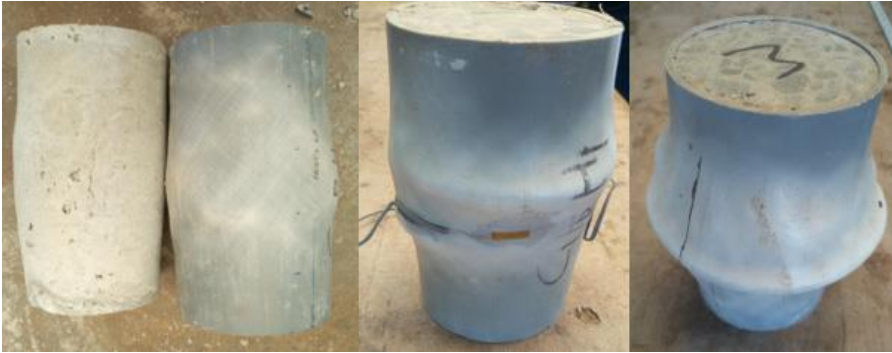
Figure 3: Shear fracture of composite specimen (Woldemariam, 2019)
