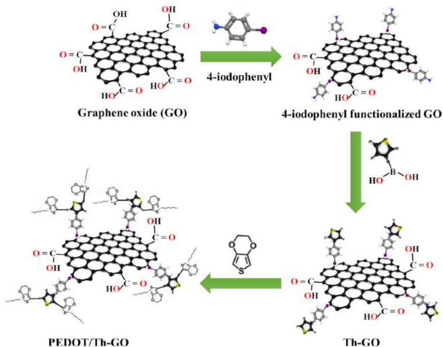
Figure 3: Synthesis illustration of GO/Th/PEDOT electrode (Wang, et al., 2015:370; Ansari et al., 2025;115564).
