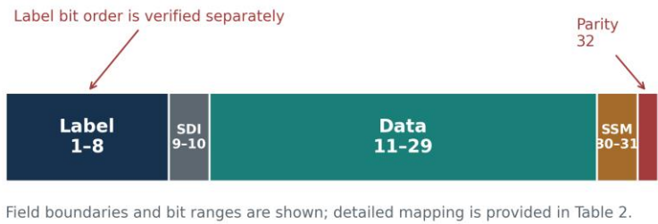
Figure 2. ARINC 429 logical word fields and bit numbers (drawn by the author based on ARINC 429P1-19).
