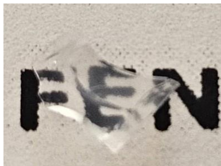
Fig. 4.3. Crystal structure appearance and transparency test of silica aerogel (16% water)
