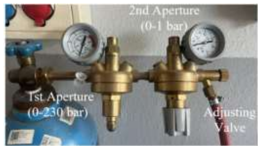
Figure 2. Dual-stage diaphragm gas regulator used for controlling molten metal movement and adjusting the applied gas pressure.
