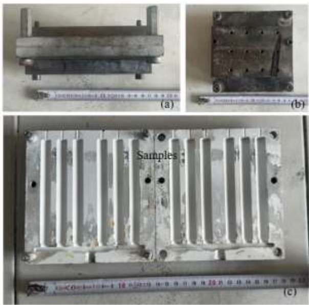
Figure 3. Top view (a), front view (b), and mold cavity view (c) of the metallic mold.
